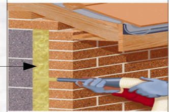
Installation of Rockwool EnergySaver into traditional brick/block cavity wall
